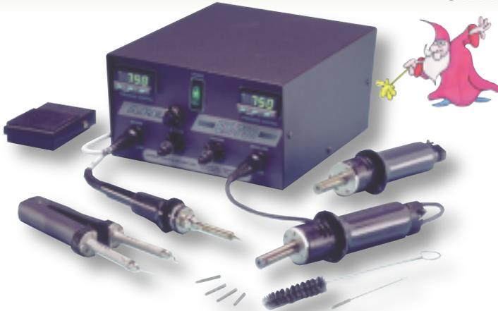
The EX-750 Rework and manufacturing system performs surface mount and conventional component repairs. Tip temperature is electronically controlled from 450 to 900°F (232 to 482°C). Two programmable digital controllers feature responsive closed-loop temperature control with large LED readouts, indicating "Set" and "Operating" temperatures.
